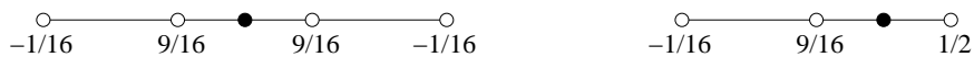
Figure 6: Stencil of 4-point curve subdivision scheme: Regular (left) and end of chain (right).
